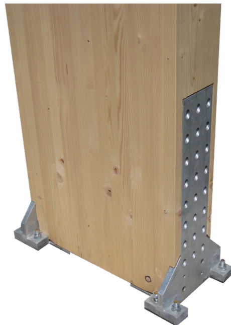
For support columns without steel plinth (interior or on concrete plinth). Connection via slanting screws, support steel part integrated in foundation with threaded rods.
