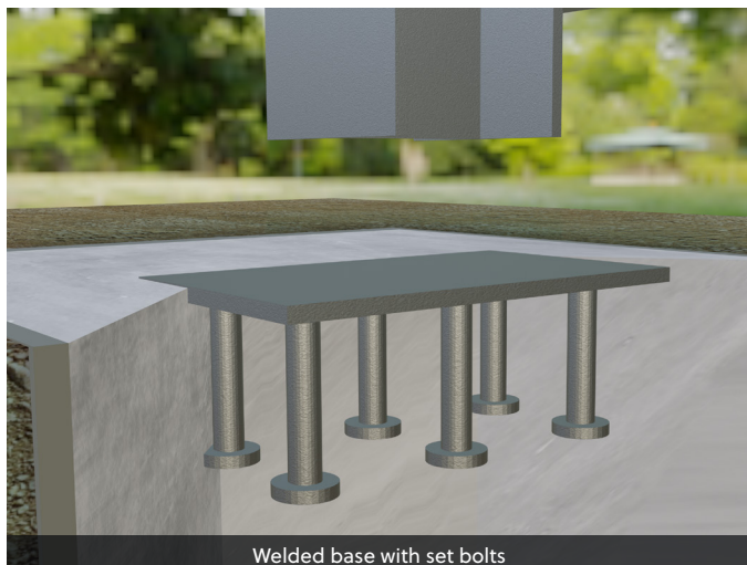
Welded base with set bolts
