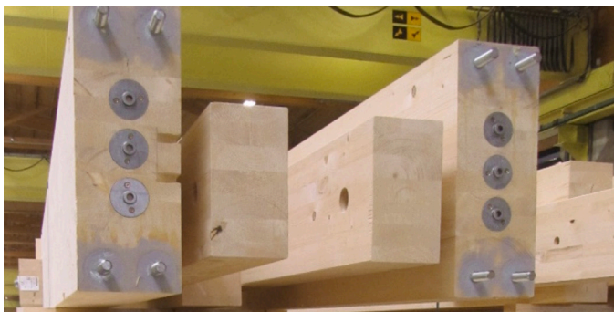
Anchor rods with thread in concrete, one-piece stanchion foot with slanting screws pre-assembled on wooden support (smaller support column widths). Wall bracing tabs possible. Structural tolerance compensation
