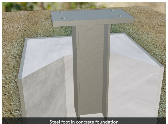
Steel foot in concrete foundation
